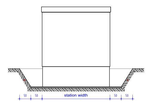
leveling layer, approx. 5cm fine chippings 2-8mm, flattened<sup>1</sup> degree of compaction of subgrade: approx. 98 %, soil pressure 150 kN/m<sup>2</sup> max. deviation regarding evenness and inclination of the fine subgrade: +/-0.5cm over the outer dimensions of the building, permissible are single imperfections up to +/-1.5cm (e.g. footprints) up to 40cm length Tolerance regarding height: according to the requirements of the customer
